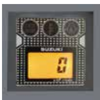
Tachometer with warning indicators
