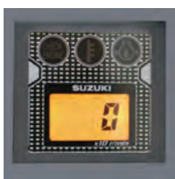
Tachometer with warning indicators
