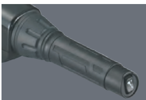
Power trim & tilt switch and throttle grip friction adjuster
